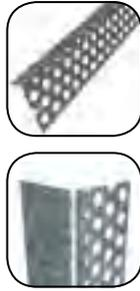
The Stopping Angle is fixed to the sheet of building board with an adhesive or staples, with the finishing coats bonding into the building board and feathering up to the bead nib. Ideal for use around door jambs, however, in this application it is recommended that when using building board up to 10mm thick, a P26 should be used so that the leg will slot into the door jamb as shown. Similarly, when using 1/2" board, P27 should be used.
