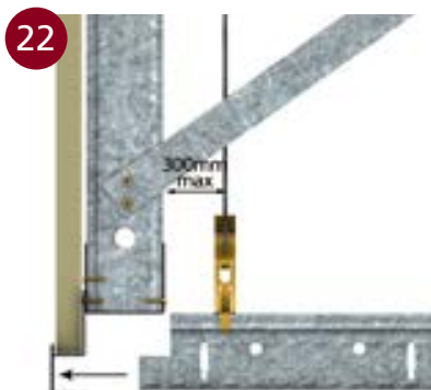
■ VERTICAL SCREW-FIX SYSTEM DETAIL
