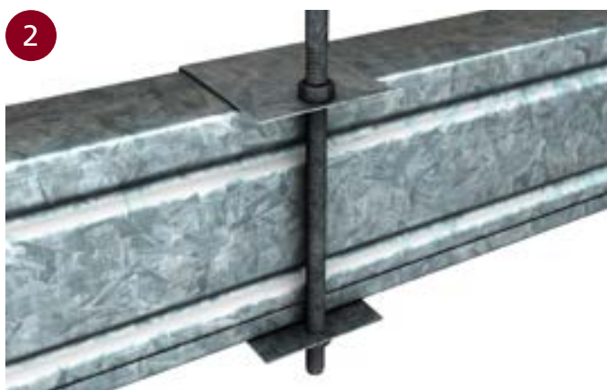
■ ATTACHING STUDS TO THE ROD
