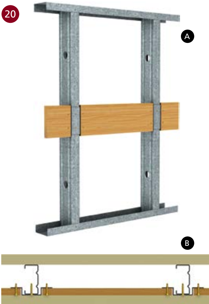
■ TIMBER NOGGINGS FITTED USING Judah CONTINUOUS NOGGING BRACKET
