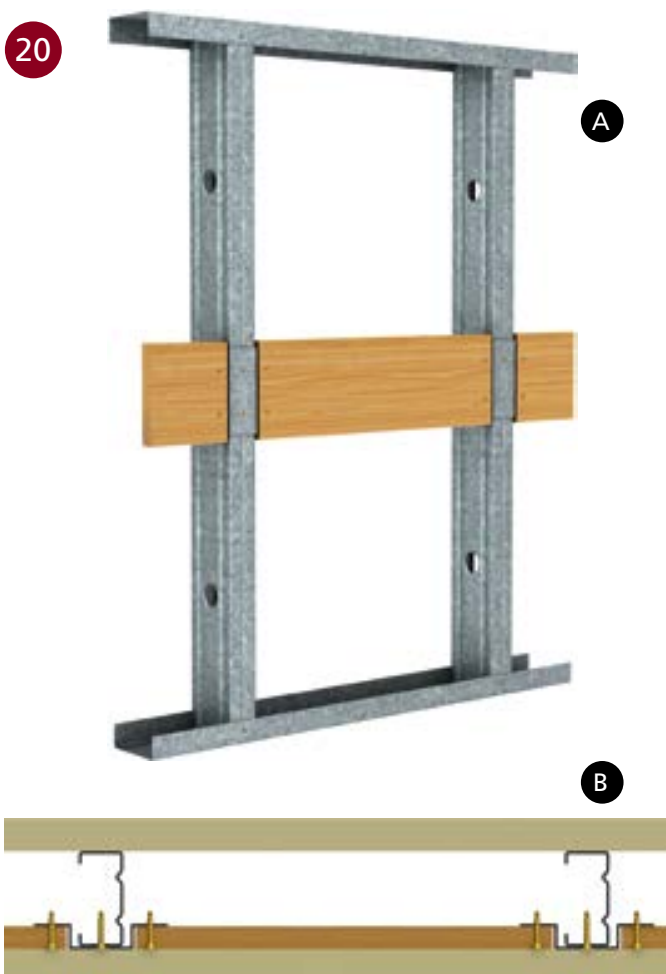
■ TIMBER NOGGINGS FITTED USING Judah CONTINUOUS NOGGING BRACKET
