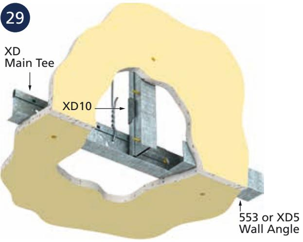
■ 90° OUTSIDE CORNER WITH MAIN TEE AT BOTTOM EDGE AND DETAIL
