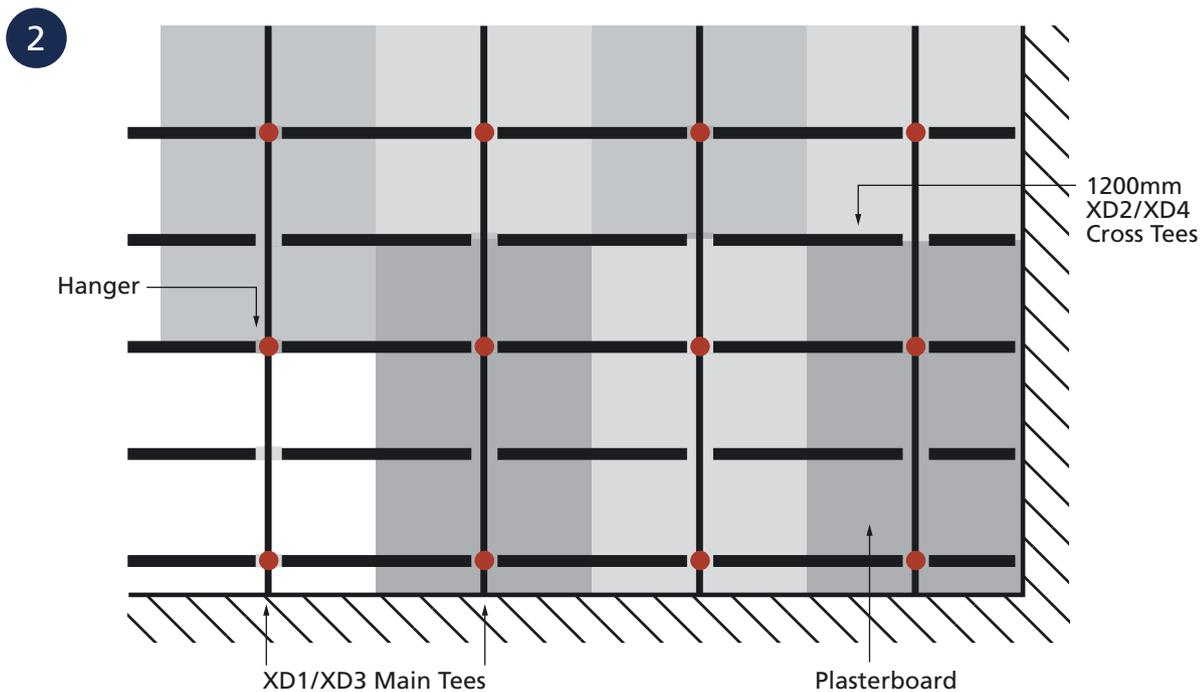
NOTE: When butt-joining on Cross Tees, it is recommended to stagger adjacent sheets for a better joint finish.
