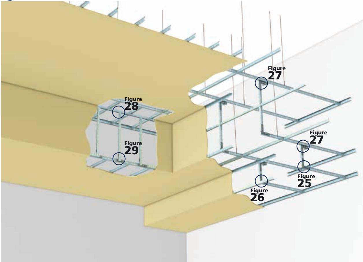
■ Judah XPRESS® DRYWALL GRID BULKHEAD/SOFFIT
