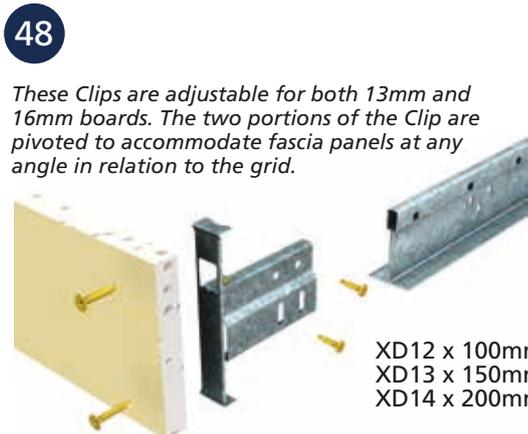
48 These Clips are adjustable for both 13mm and 16mm boards. The two portions of the Clip are pivoted to accommodate fascia panels at any angle in relation to the grid.
