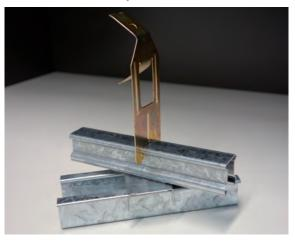
When using the Judah 238 Swivel Clip, the Furring Channel can be rotated 360 degrees, therefore enabling any Furring Channel set out required. The span of the Furring Channel between these attachment clips should not exceed the recommendations in Rondo's Professional Design Manual.
